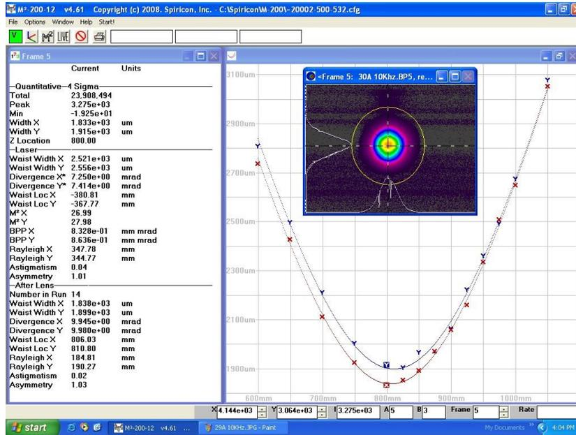
Myron-HP-532-M Output Beam M<sup>2</sup> Measurement
